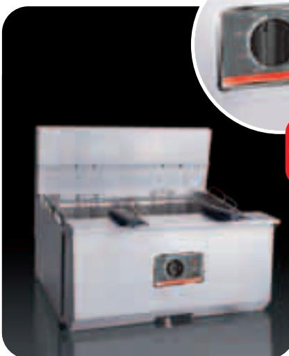
**E** Single vat table top fryer. Integrated fat melting cycle. Precise temperature control of +/- 1°C. Oil content 12 - 15 liters. Output per hour 20 - 25 kg. Two frying baskets, max. load 0,75 kg, recommended load 0,5 kg per basket.
