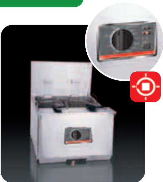
**E** Single vat table top fryer. Integrated fat melting cycle. Precise temperature control of +/- 1°C. Oil content 8 - 9,5 liters. Output per hour 19 - 22 kg. Available with one large or two small frying baskets.
