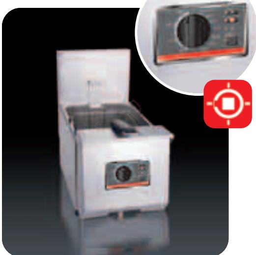
**E** Single vat table top fryer. Integrated fat melting cycle. Precise temperature control of +/- 1°C. Oil content 5 - 7 liters. Output per hour 12 - 14 kg. Delivered with one frying basket.
