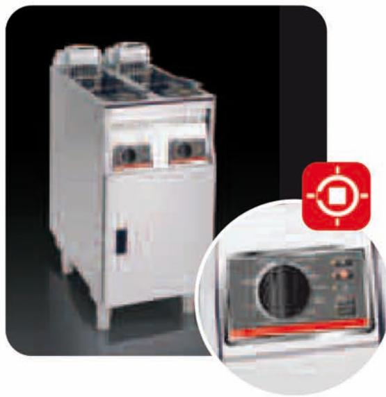
E Split vat fryer with an easy to operate control panel per vat. Integrated fat melting cycle. Precise temperature control of +/- 1°C. Oil content 2 x 7,5 - 9 liters. Output per hour 2 x 17 - 22 kg. Two frying baskets, max. load 1,25 kg, recommended load 0,9 kg per basket.
