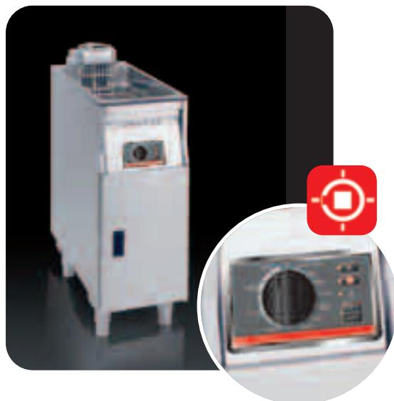
**E** Full vat fryer with an easy to operate control panel. Integrated fat melting cycle. Precise temperature control of +/- 1°C. Oil content 12,5 - 14,5 liters. Output per hour 27 - 32 kg. One or two frying baskets, max. load 1,5 kg, recommended load 1 kg per basket.
